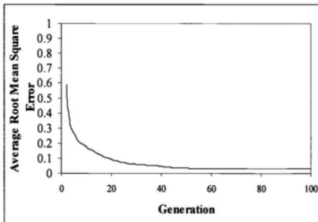
Fig. 2. Rapid convergence of the genetic algorithm when performing a test search for the Bernoulli equation
