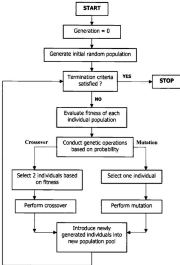
Fig. 1. Flowchart for the genetic algorithm
